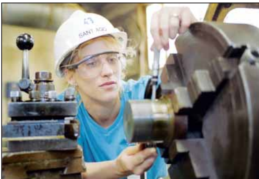
Newport News Apprentice checking diameter during machining process. Newport News Photo
