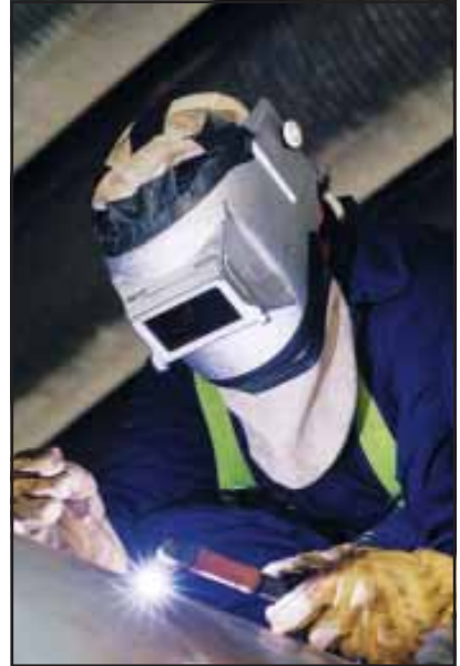
Newport News Welder Using the TIG (Tungsten-Inert-Gas) welding process.
